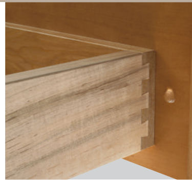
DOVETAIL DRAWER WITH 3/4" NOMINAL THICK ALL-WOOD SIDES & FULL EXTENSION GUIDES
